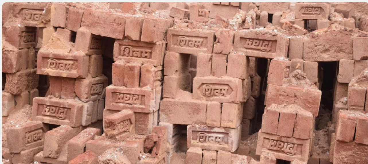
Bricks arranged in a zigzag pattern in the kiln. This increases the length of the airflow path, improving combustion and heat transfer rates. Image by Manish Chandra Mishra/Mongabay.
